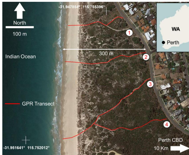
Figure Error! No text of specified style in document..3: Location and orientation of the ground penetrating radar (GPR) transects featured in this paper. Shallow geology is described predominantly Tamala Limestone and Safety Bay sands. Total perpendicular length from the coastline is approximately 300 m.
